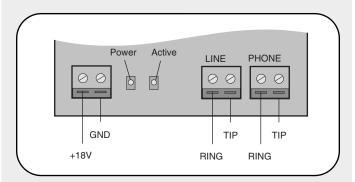
Use the supplied Test/Program Cord for programming and testing before completing connections to phone company's d-mark box.
